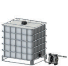
Pump installed below head (positive suction)
